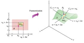
Each side of  $\Delta A_{uv}$  maps to a curve on the surface S, and together these four curves bound a "curved area element"  $\Delta \sigma_{uv}$ .
